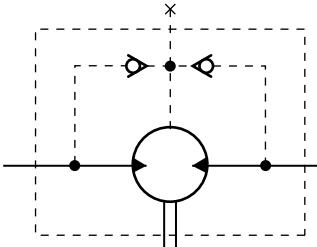
In applications without drain line, output shaft seal exceeds a bit of the pressure in the return line. When applications use the drain line, the pressure of output shaft seal equals the pressure in drain line.
