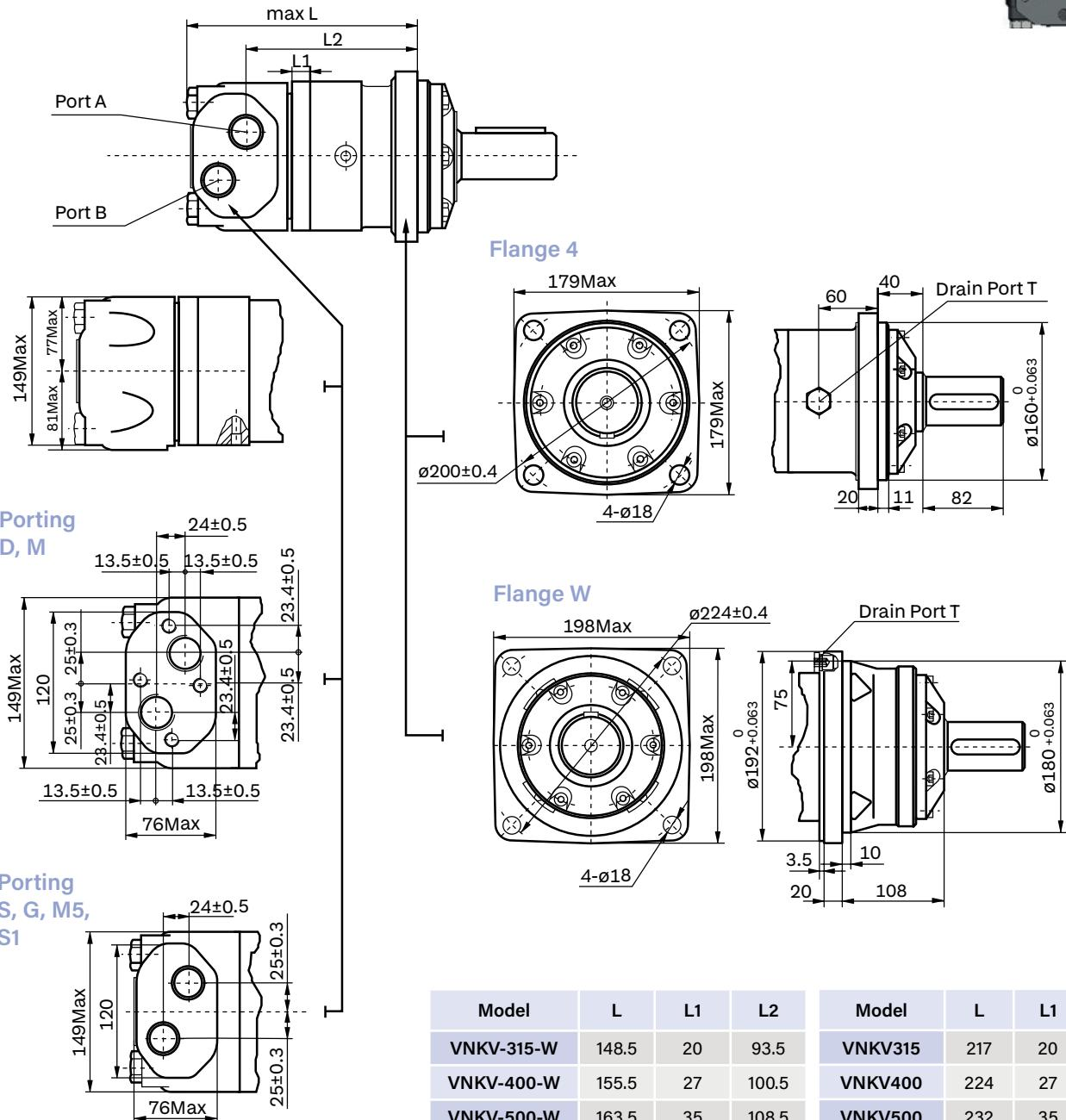
**Note:** The thickness of the stator and rotor is the dimension of L1 adding on 7mm.
