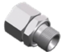
RACOR HEMBRA GIR. DKO MACHO BSPP C/ JUNTA FKM AISI 316L SWIVEL DKO FEMALE FITTING BSPP MALE WITH FKM SEAL RACCORD FEMELLE TOURN.DKO MÂLE BSPP A/JOINT FKM AISI 316L
